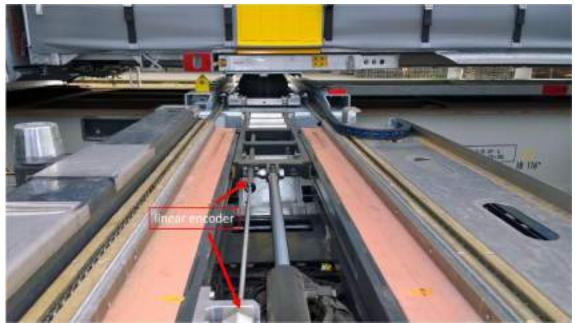
Figure 14 – the linear encoder for measuring the exact distance the contract bridge is ejected.
