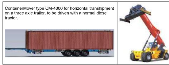
Figure 37 - ContainerMover-4000 and Reach Stacker
