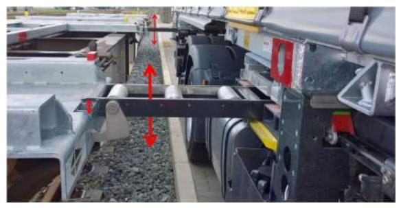
Figure 16 – Adjusting the height of the two "contact bridges"
