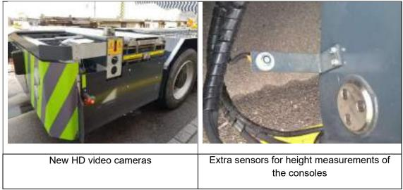
Figure 25 – HD Cameras and ultrasonic sensors (Picture InnovaTrain)
