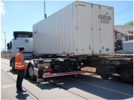
Figure 1 – ContainerMover 3000 controlled by wireless remote control
