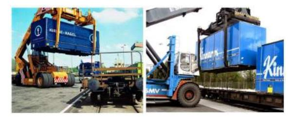
Figure 30 – reach stacker using crappler arms for a swap body Source: http://the-mediarail-chronicles.blogspot.com
