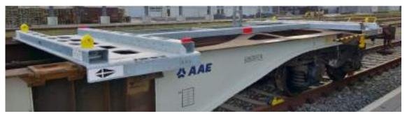
Figure 3 – Wagon adaptor frame on 20' position
