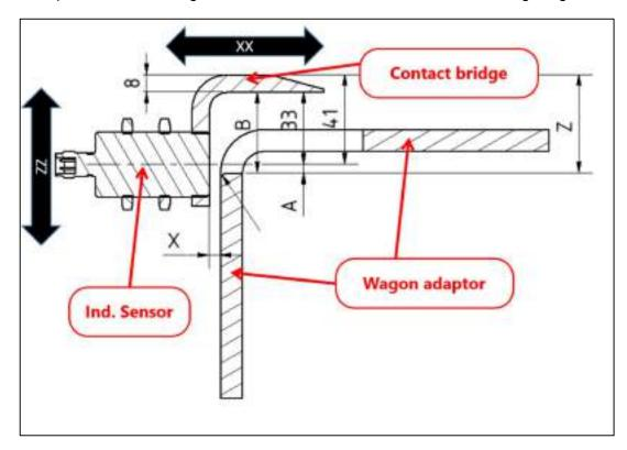
The tip of the contact bridge was then moved in X and Z direction, according to figure 33:
