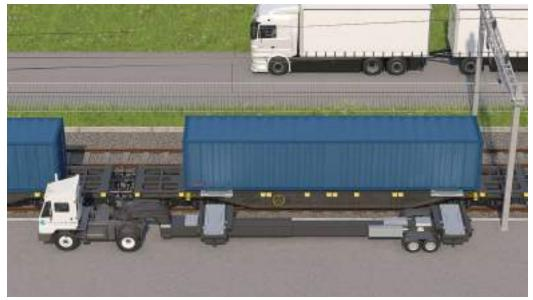
Figure 6 – CM-4000 for weights up to 35 tons (45' container)
