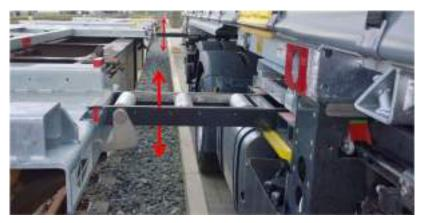
Figure 32 - Adjusting the height of the two "contact bridges"
