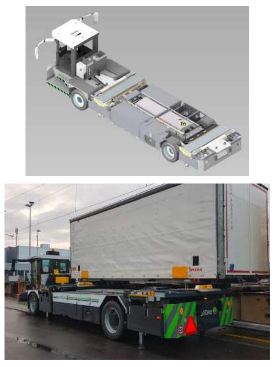
Figure 24 – Container Mover 3040 (Picture railCare)
