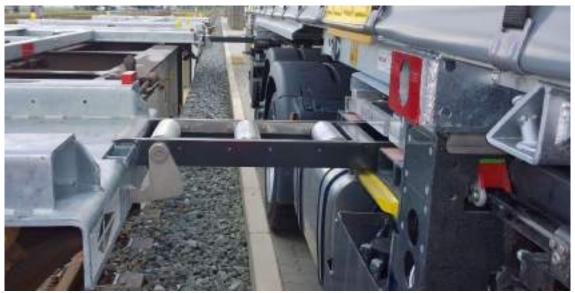
Figure 15 – The contact bridge between ContainerMover and Wagon Adaptor
