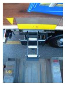
Figure 5 – The two "contact bridges" between truck and railway wagon
