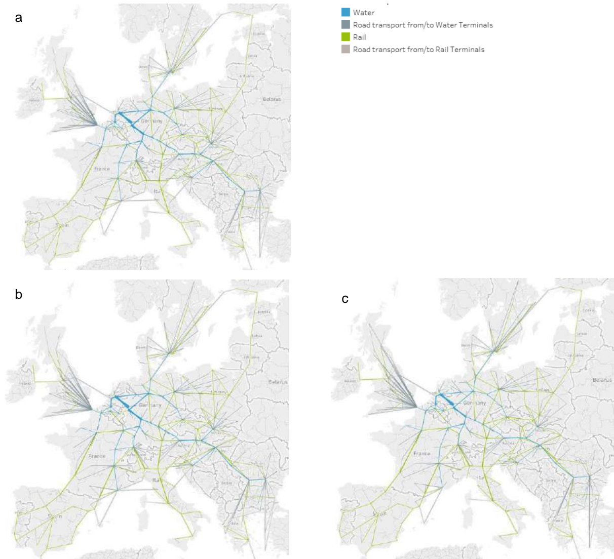
Figure 17: Network paths per for each modal shift scenario a. Modal shift of road transport >300 km b. Modal shift of road transport >700 km c. Modal shift of 50% of ton kilometres of road transport >300 km
