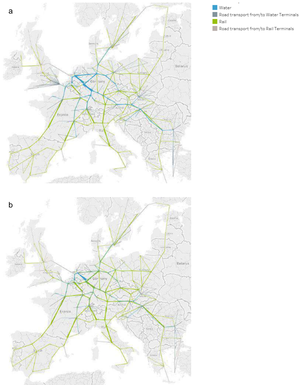
Figure 22: Network paths per for each CO 2 emission minimisation scenario a. Maximum allowed CO 2 emission is 60 billion kgs b. Maximum allowed CO 2 emission is 55 billion kgs
